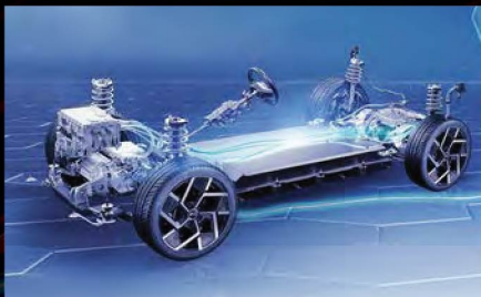
Safety - E-Platform 3.0 With The Cell-to-Body (CTB) Structure
